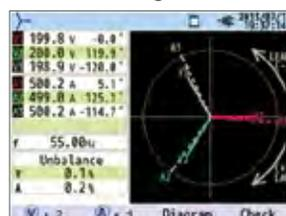
**Configure advanced functions** such as nominal voltages and transient limits or check for available memory by pressing the SET UP button
