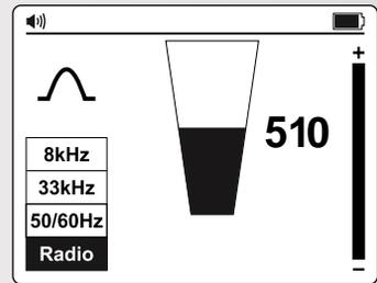
Passively locate any utility, Energized or De-energized, with **Radio Mode**
