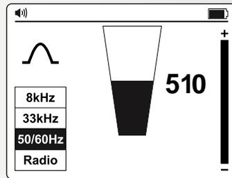
Passively locate Energized cables and power lines with **Power Mode**
