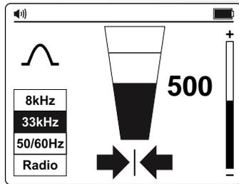
In an **Active Mode** using the Transmitter, arrow indicators help quickly assess the location of the utility
