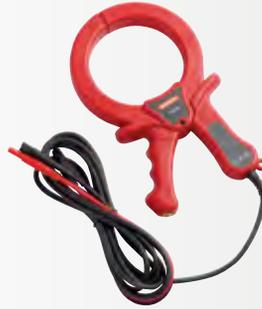
**SC-600 Signal Clamp** The Signal Clamp accessory provides an efficient and safe method of applying a locate signal to a cable, enabling the Transmitter to induce a signal through the insulation into the wires or pipes. The clamp works on low impedance closed circuits only.
