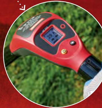
..... Detect ground faults on cables and pipes
