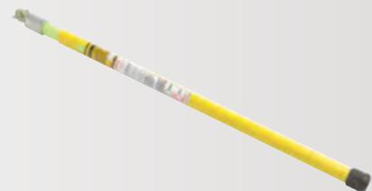
**TIC-410A Hot Stick Attachment** extends the reach of the TIC 300 Pro high voltage detector for checking transmission lines, power distribution equipment, down power lines, fuses, and load break connectors. Extends the voltage limit on the TIC 300 Pro from 1500 AC to 122,000 V AC (122 kV) and adjusts from 33" to 57". Just screw it onto the universal adapter on the TIC 300 Pro high voltage probe — no other tools are required.
